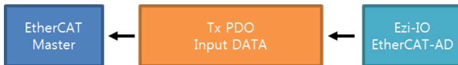
Figure 7-2. EtherCAT PDO Communication
