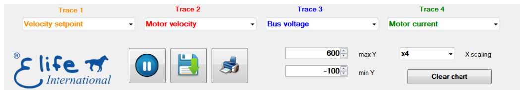
Figure 4.3: Telemetry Panel allows you to plot and log one or more telemetry data.
