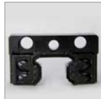
End seal in good condition
